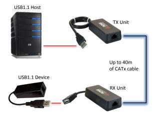
Cable requirements The CATx extension cable can be CAT5e, 6, or 7 UTP/STP cable. The CrystalLink USB1.1 performs best with solid core cable. Stranded (patch) cable and the use of patch panels will reduce the maximum operational distance. STP cable with grounded metal hoods is recommended. Do not use CrystalLink USB1.1 between buildings or for outdoor extension requirements.
