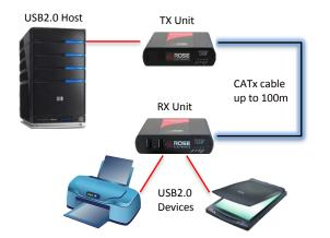
The CrystalLink USB2.0 dual-port is ideal for use in commercial, industrial, residential, medical, data center, and other environments where USB devices need to be connected at distances up to 330 feet (100m) away from a host PC.
