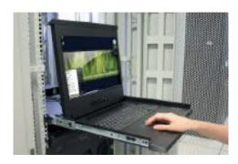
**Installation** RackView High-Res is very easy to install. Simply adjust the rack-rail length to the depth of your rack, slide the unit through the rack and secure the rack mount brackets to the front and rear rack rails.
