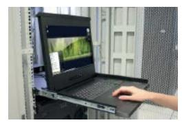
**Installation** RackView Widescreen is very easy to install. Simply adjust the rack-rail length to the depth of your rack, slide the unit through the rack and secure the rack mount brackets to the front and rear rack rails.
