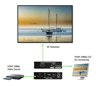
**Installation** This product is quick and easy to install. Power off all the video sources and monitors, then connect the HDMI cables from the HDMI 4K2K Scaler to the peripherals. Set the bypass switch for video upscale or video downscale. Next, power on the HDMI Scaler, followed by the monitor and the video sources. When the input video signal is detected, the corresponding LED will illuminate.
