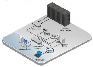
Models The UltraConsole Remote 2 is available in several models. They have fixed port configuration and plug-in expansion cards. There are models that connect a user to 4, 8, or 16 computers. Adding expansion units can expand the system to as many as 1,000 computers or serial devices.
