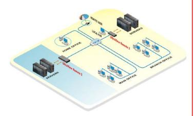
UltraView Remote 2 Model The UltraView™ Remote 2 is available in an 8, and 16 port version. UltraView Remote 2 can be chained together with our UltraView Pro or ServView Pro to support up to 256 computers.
