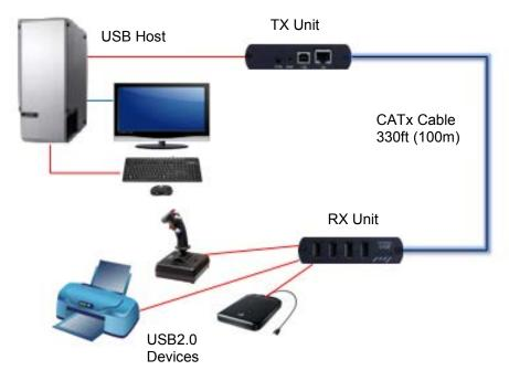
Figure 4. CrystalLink USB2.0 CATx extender – standard installation
