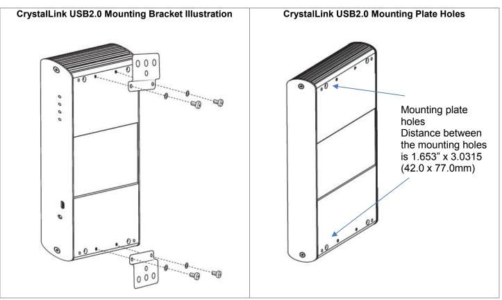
Figure 5. Chassis mounting options
