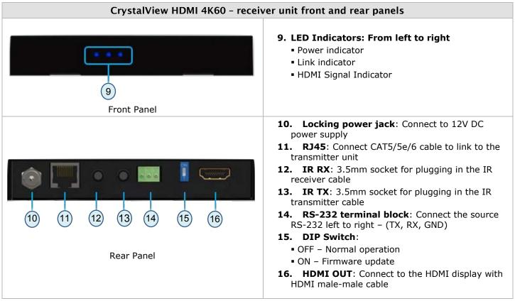
Figure 2. Receiver front and rear panels
