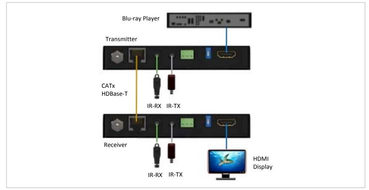
Figure 3. CrystalView HDMI 4K60 – installation diagram
