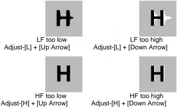
Figure 12 HF / LF adjustment guide.
