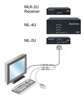
Figure 7. Connecting the KVM
