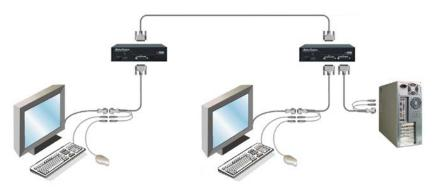
Figure 9. Connecting Bus Cable
