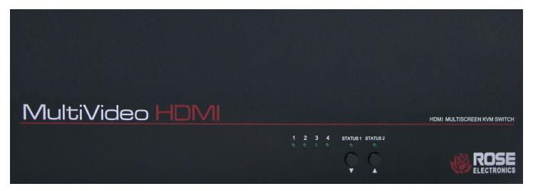
Figure 3. MultiVideo HDMI Quad Front Panel
