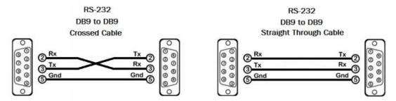
Figure 7. Examples of 9 pin RS-232 Straight Through and Crossed Cables
