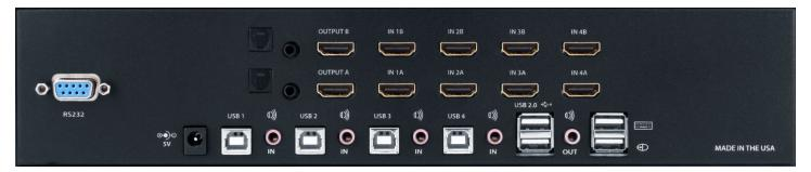
Figure 2. MultiVideo HDMI Dual Rear Panel
