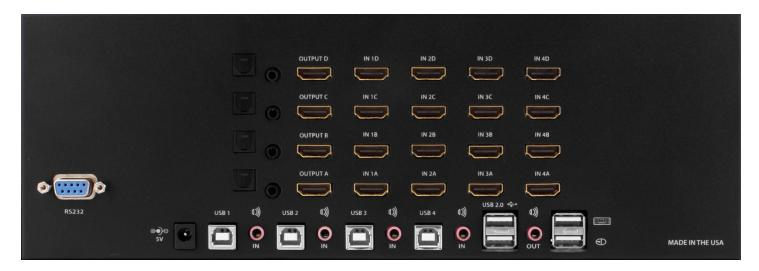
Figure 4. MultiVideo HDMI Quad Rear Panel
