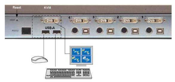
Figure 3. Local KVM Console Installation
