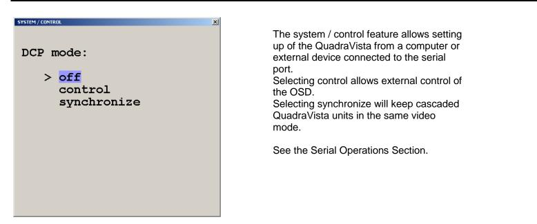
The DCP (Device Control Protocol) offers three modes, off, control and synchronize. Set the DCP mode to "Control" if a single QuadraVista 2 will be controlled from an external computer. Set the mode to "Synchronize" if you system features several linked QuadraVista 2's. When in this mode the QuadraVista 2 status is transmitted to the external computer. For local unit operation, set the mode to off. See the **Serial Operations** section for detailed information on the DCP mode.
