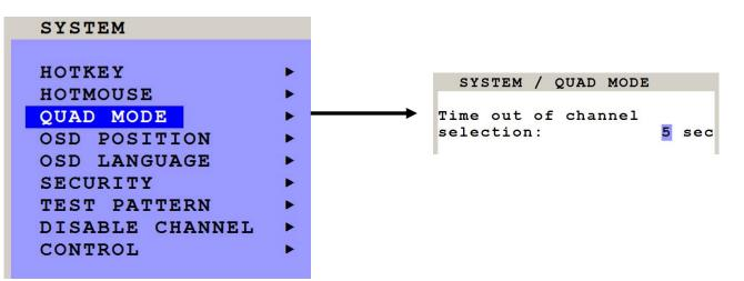
Channel selection timeout defines the period (1 to 30 seconds) after which the selector will close automatically. Default setting is 5 seconds.
