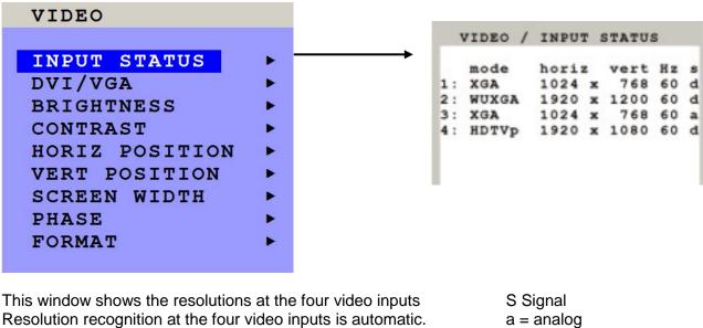
Some analog input resolutions may not correctly be detected.
