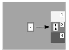
Activating the Hotmouse in the Quad screen mode will display a box cursor with the active channel number in the box (see below). Moving the cursor to any quadrant and clicking on the left mouse button will switch control (keyboard / mouse) to that channel.
