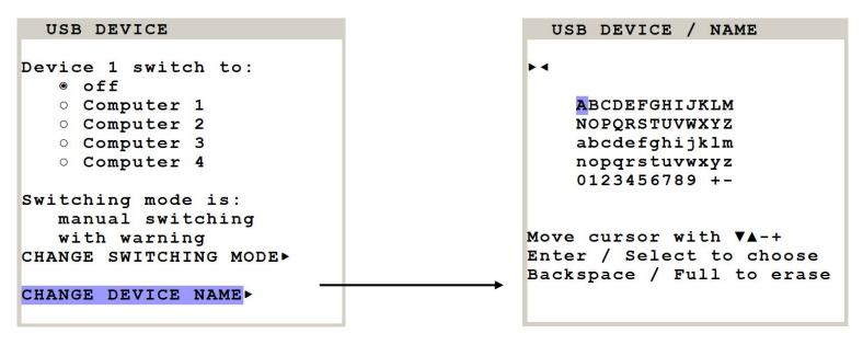
**Note:** Use hotkey + "u" (by default: hotkey = Ctrl + Alt) to quickly access the USB DEVICE 1-4 menu. This allows quick access to this menu when switching manually. To directly open the switching menu of e.g. USB device/port 1 use hotkey + "F1" (by default: hotkey = Ctrl + Alt).
