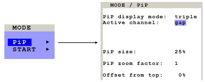
In the PIP window you can configure PiP size, position, and display mode.
