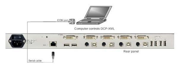
Use the serial cable to connect the COM port of the Windows computer with the serial port of your QuadraVista 2.
