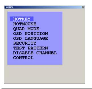
The system Menu is called up by highlighting SYSTEM from the main menu and pressing enter. From the system menu you can set-up:
