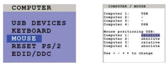
The upper half of the MOUSE window shows which mouse type (USB, PS/2 or PS/2 wheel) has been recognized at which computer port.
