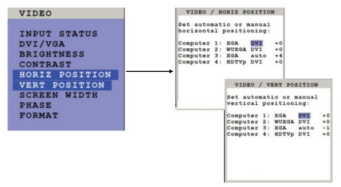
In case of incorrect horizontal position of a computer screen, use this feature to adjust the computer screen manually. Use the arrow keys to navigate to the AUTO/MAN field and set MAN for manual. Use the "+" or "-" keys in the value field to adjust the vertical position between –20 and +20, and the horizontal position between –63 and +63.
