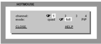
In the Full screen or Quad mode, the Hotmouse menu allows you to switch channels, change display modes (quad, full, PiP, Dual), or activate a channel.
