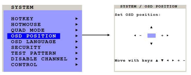
The will set the OSD position. Use the UP / DOWN / LEFT / Right / + / or - key to position the OSD window to any position on the screen
