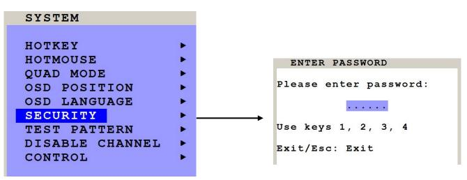
The SECURITY feature allows you to reduce the functional range of QuadraVista 2. Eight security levels are available for this purpose.
