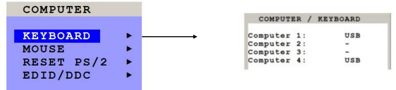
Use this display feature to identify which keyboard type (USB, PC1, PC2 or PC3) has been recognized at which computer port.
