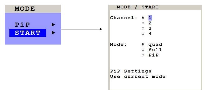
This feature allows you to define the start configuration, i.e. the display mode (Quad, Fullscreen, or PiP), active channel, and PiP settings which QuadraVista 2 uses after a reset or when the system is powered up.
