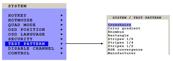
Use the Test Pattern to check the function of internal video circuits or to check the quality of the connected console monitor. It's recommended to use all the test patterns for the test procedure.
