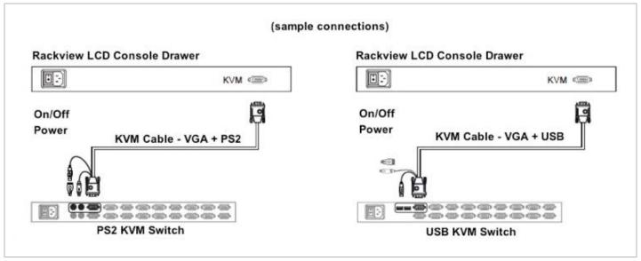
Figure 8. RackView cable connectivity
