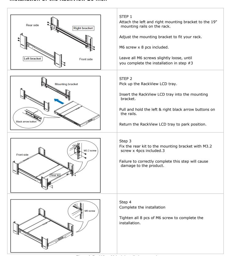
Figure 6. RackView 20-inch installation procedure
