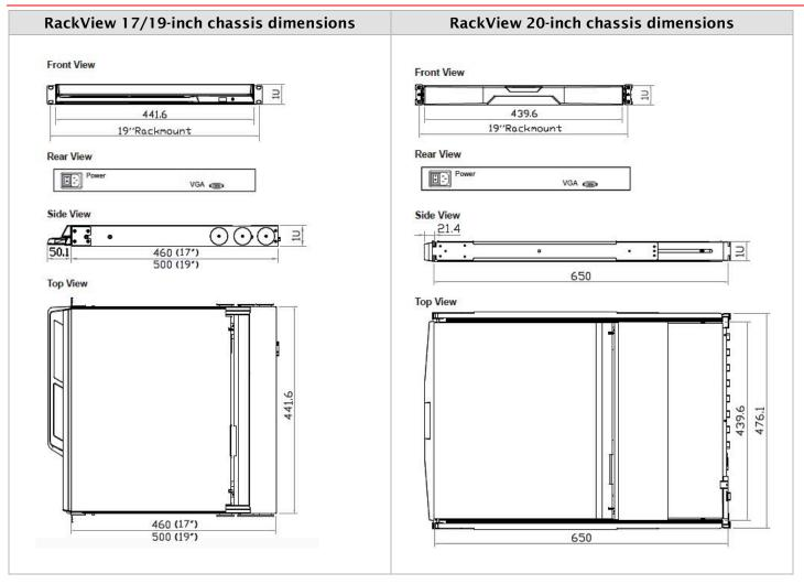
Figure 4. RackView chassis dimensions
