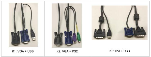
Figure 8. RackView device interface cables
