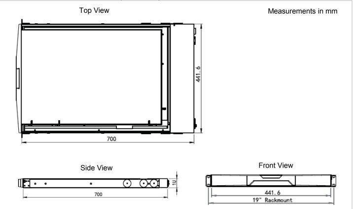
Figure 14. RackView chassis dimensions (24" model)
