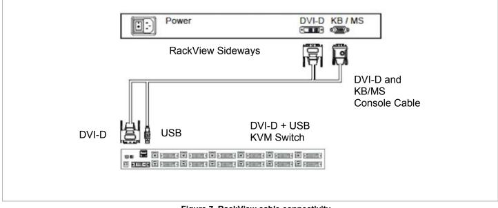
Figure 7. RackView cable connectivity
