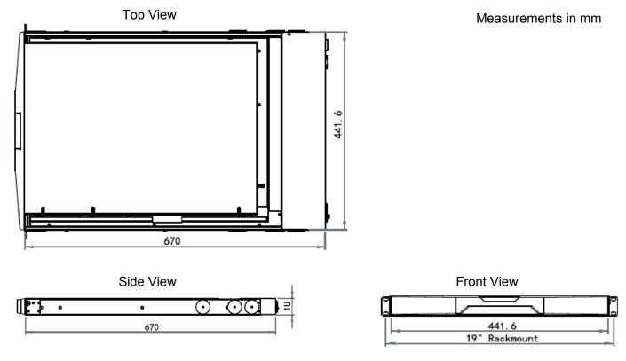
Figure 13. RackView chassis dimensions (21" model)
