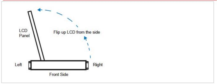
Figure 4. RackView with left-side or right-side opening
