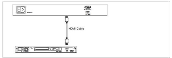
Figure 17. HDMI cable connection
