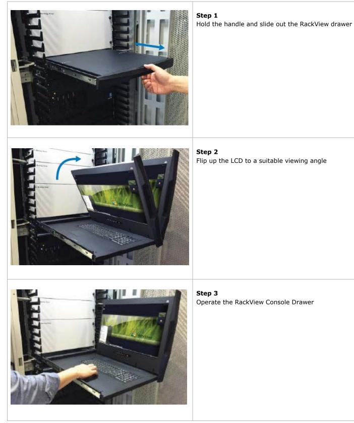
Figure 6. RackView console drawer operation
