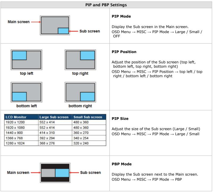
Figure 11. PIP and PBP configuration
