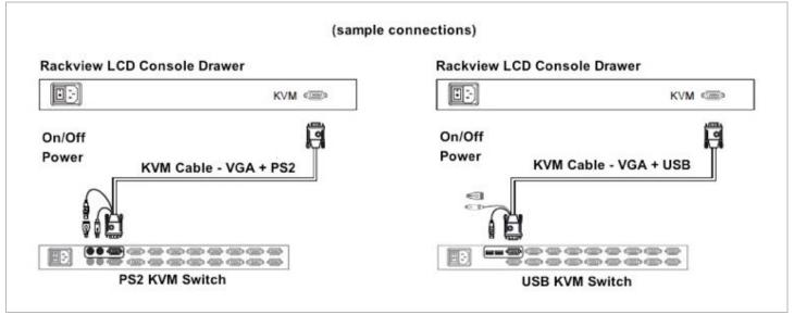
Figure 5. RackView cable connectivity
