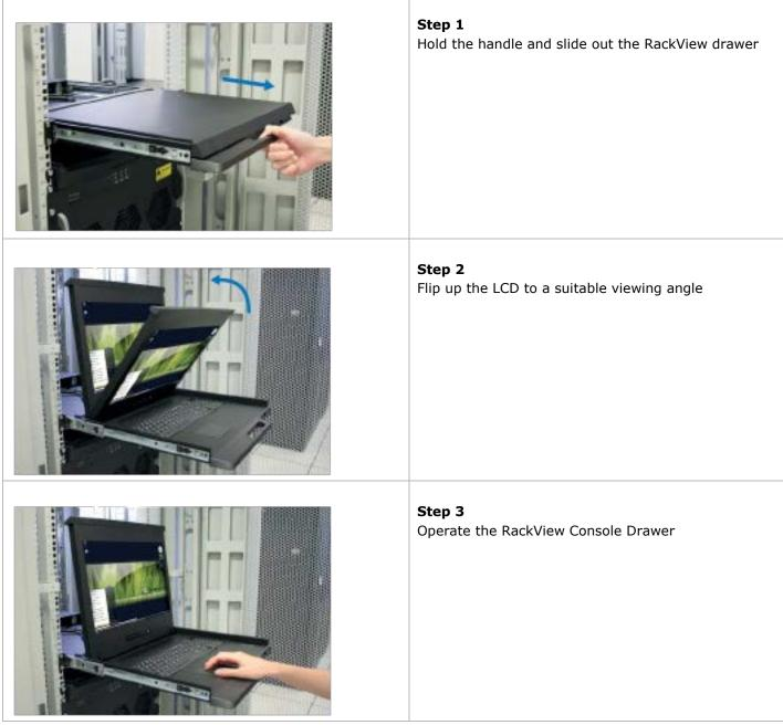
Figure 4. RackView console drawer operation
