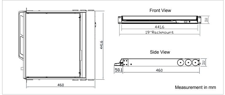
Figure 9. RackView chassis dimensions
