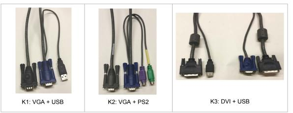
Figure 6. RackView device interface cables
