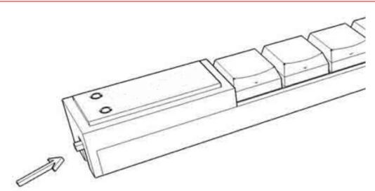
The programming switch is located on the left side edge of the 4/8/16 Keystick. The program switch will display the MacroWorks GUI by default. If desired, the program switch can be used like any other key on the RCK-Keystick, effectively making it a 25 button device.
