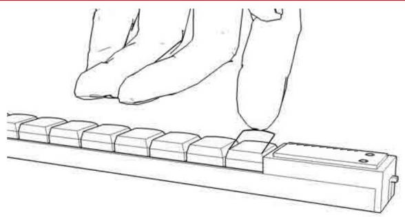
Labels may be inserted under the clear lens, which can be removed by prying with a fingernail or other thin object. Additionally, custom keycaps and lens are available.
