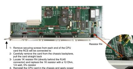
Figure 1. Replacing Resistor R4
