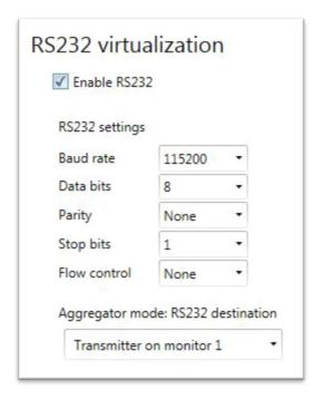
Figure 15. RS232 Virtualization on the Receiver
