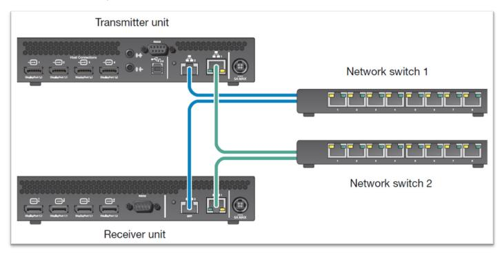
Figure 19. Connecting Transmitters and Receivers to Support Link Redundancy
