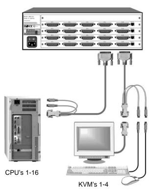
Figure 4. Installation - Single unit
