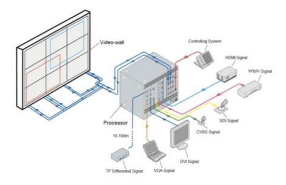
Figure 10. System Diagram of UltraVista Pro
