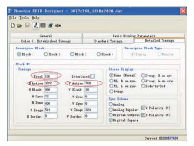
Figure 29. Modifying the Screen Resolution Using the EDID Editor
