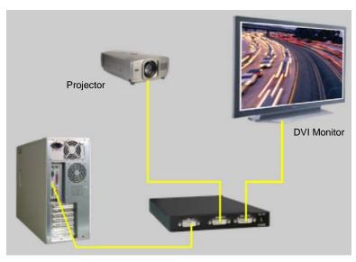
Figure 2. Basic Installation
