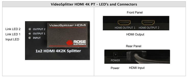
Figure 3. Description of LED's and Connectors
