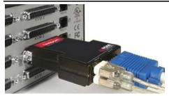
Connect the DB25M connector to the DB25F KVM port on a Rose KVM switch. Next connect your USB keyboard and mouse to the USB Type A connectors on the Uniport. Connect the video cable (HD15M) to the Uniport's HD15F connector.
