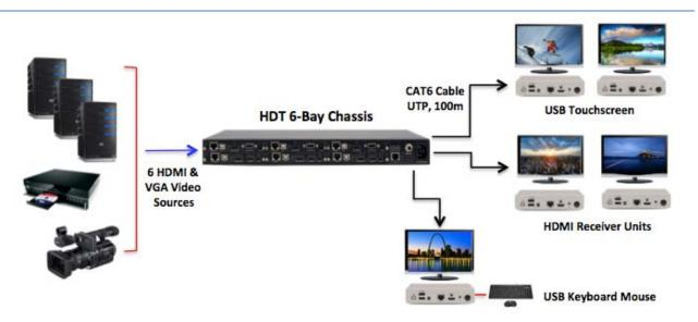
CrystalView HDT set-up when connecting to multiple video sources
