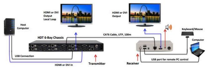
CrystalView HDT set-up when connecting to a host computer
