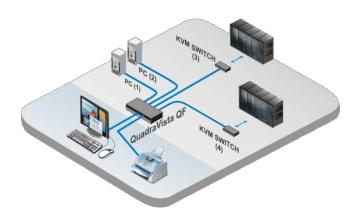
**Installation** QuadraVista 2 is easy to install. Simply connect up to four computers and a user station to the QuadraVista 2 ports. Access the onscreen menu with a simple keystroke, configure each computer connection for VGA or DVI and save it in flash memory.
