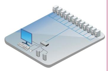
Installation Make certain that all computers and the Vista LC DVI are powered off. Connect the CPU cables between the switch and each computer using the Vista LC combo cables. Connect the DVI monitor and the USB keyboard and mouse to the local port connectors on the switch. If you're using a stereo audio speaker, connect that as well. Power on the system in the following sequence: first the display, then the Vista LC DVI switch, followed by the individual computers.
