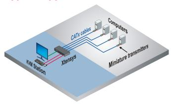
The Xtensys Mini CATx KVM Switch is suitable for industrial environments, computer test environments, production lines, data centers, and other applications. Automatic video equalization and skew compensation ensures the clearest possible video image up to a maximum cable length of 1000 feet.
