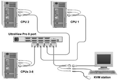
(4 CPUs can be connected using a 4-port unit, 16 using a 16-port unit)
