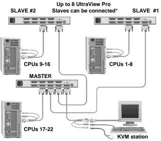
\* 4 units can be cascaded using a 4-port master/16 using a 16-port master
