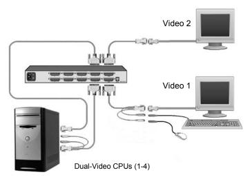
Figure 3. 4U2V Unit installation
