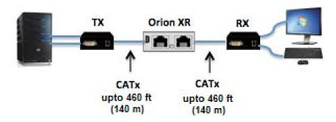
Figure 2. A Single CATx/CATx Repeater Doubles Extension Distance
