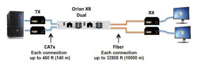
Figure 4. Dual CATx/Fiber Repeater Allows One Unit to Connect Two Sets of Extenders
