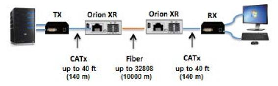
Figure 3. Two CATx/Fiber Repeaters Allow Extension to Greater Distances
