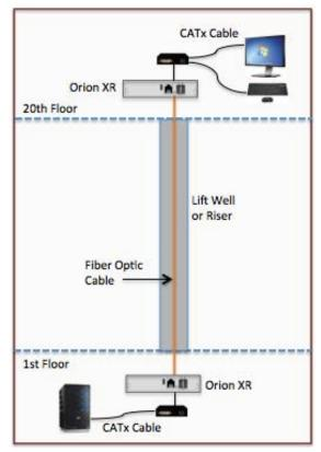
Figure 1. Cross-conversion of CATx and Fiber Signals Allow Extension to Great Distances
