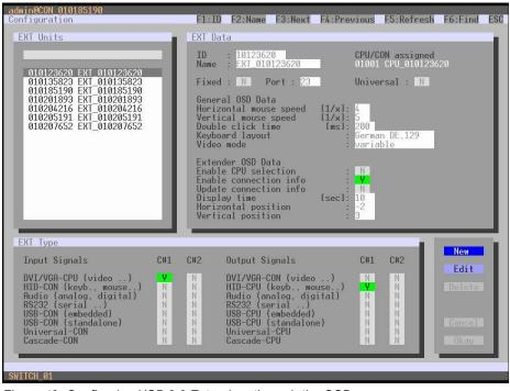
Figure 49. Configuring USB 2.0 Extenders through the OSD
