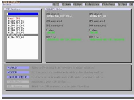
Figure 91. CON Switching Through the OSD
