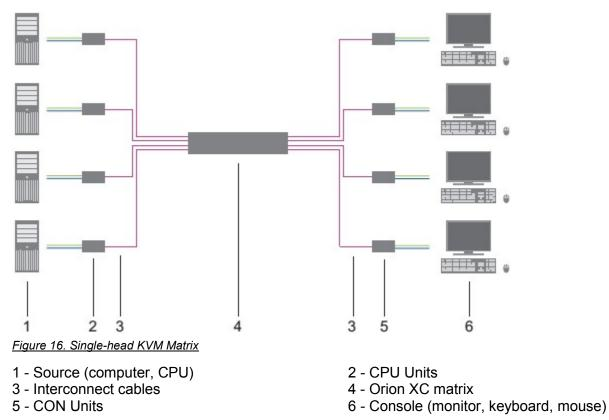
If a single-head console is used, it is also possible to access a dual-head or quad-head computer, but control is only possible at monitor 1.
