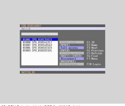
Figure 87. CPU Selection List in OSD for KVM Switching
