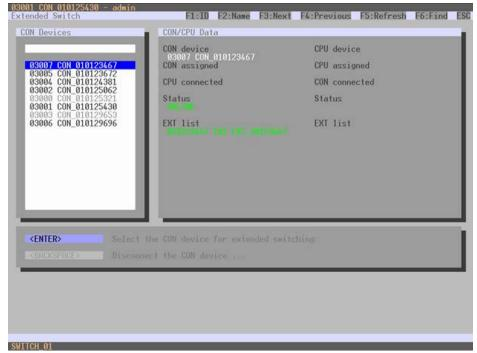
Figure 88. Extended KVM Switching through the OSD
