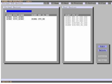
Figure 25. Virtual CPU Devices Assignment through the OSD
