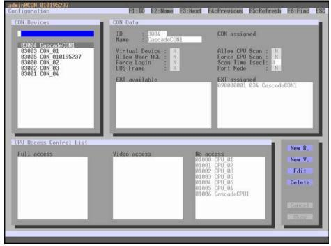
Figure 53. Setting Up CON Devices through the OSD
