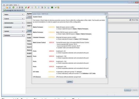
Figure 110. System Check through the Java Tool
