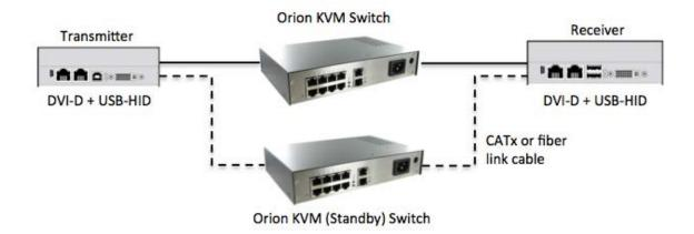
Orion XTender models with the redundant port configuration include the VGA, DVI-D, HDMI, DisplayPort and SDI video interfaces. The redundant port link cable can be either CATx or duplex LC fiber. When connected via a standby Orion KVM switch, the redundant port XTenders provide a backup link in the event of unavailability of the primary Orion KVM switch.
