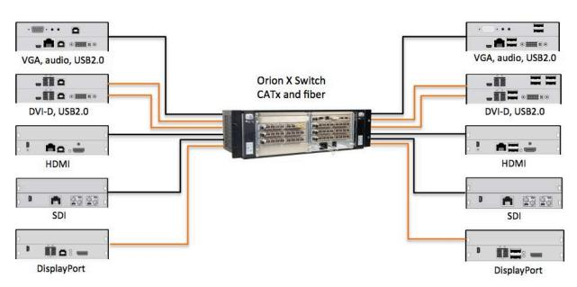
The Orion digital KVM switching system supports a mix of CATx and fiber link cables. Orion XTender Transmitter and Receiver units supporting different video interfaces (VGA, DVI-D, dual-link, HDMI, DisplayPort 2K/4K and SDI) are connected to the Orion KVM switch. Single-link video interfaces are interchangeable, for example, VGA input to DVI-D output, or HDMI Input to DisplayPort output.
