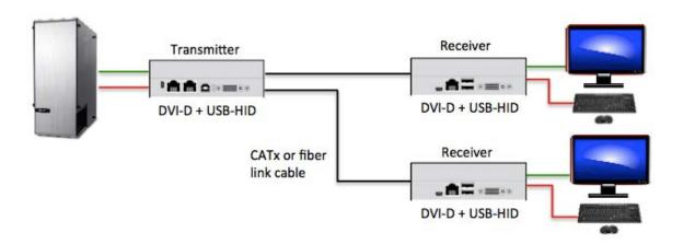
The Orion redundant port XTender product splits the video, USB-HID and peripheral data signals into two output signals. These signals can be connected using either CATx or duplex LC fiber cable to two receiver units. This enables two remote users at different locations to access the same host PC. Contention for control of the host PC is governed by keyboard inactivity timeout.
