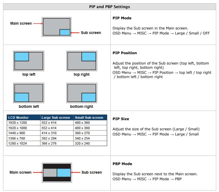
Figure 7. PIP and PBP settings and operation
