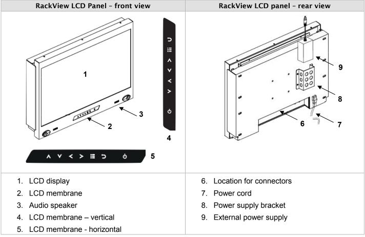
Figure 1. RackView LCD Panels - front and rear layout
