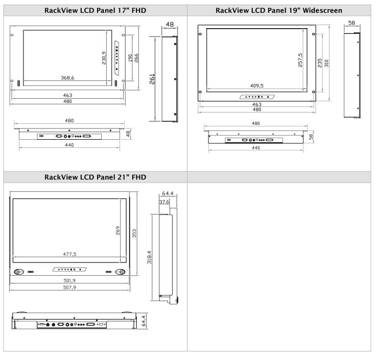
Figure 3. Chassis dimensions and LCD panel graphics
