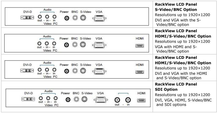
Figure 11. Back panel of the RackView LCD Panel showing standard and optional connectors
