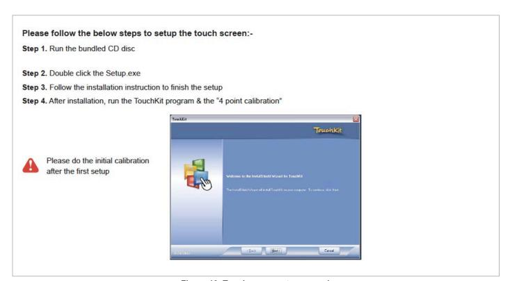
Figure 10. Touchscreen setup procedure
