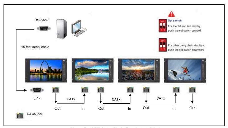
Figure 13. Multi Display Controller - Installed System
