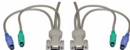
High resolution Vista cable – Computer to switch
