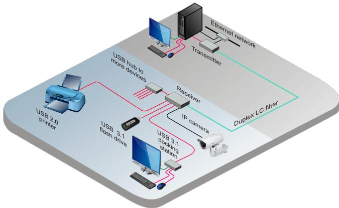
**Installation** Connect the transmitter to your computer or host device USB port. Connect the peripheral USB devices to the receiver unit. If there are more than four USB devices to connect, use a powered USB hub to expand the number of remote USB ports. Connect the transmitter to the receiver with up to 656ft (200m) of multimode fiber optic cable. Use of fiber patch cables may reduce the operating performance of the product. Apply power and the installation is complete.
