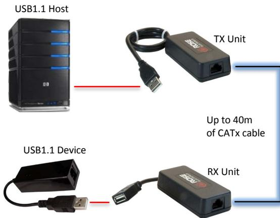
**Cable requirements** The CATx extension cable can be CAT5e, 6, or 7 UTP/STP cable. The CrystalLink USB1.1 performs best with solid core cable. Stranded (patch) cable and the use of patch panels will reduce the maximum operational distance. STP cable with grounded metal hoods is recommended. Do not use CrystalLink USB1.1 between buildings or for outdoor extension requirements.
