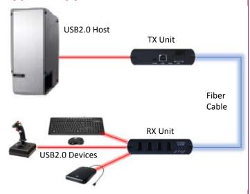
The CrystalLink USB2.0 Fiber is ideal for use in commercial, industrial, residential, medical, data center, and other environments where multiple USB devices need to be connected at distances up to 6.2 miles (10km) away from a host PC.
