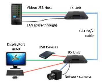
Installation Connect the host device DisplayPort video output and one of its USB 3.1 ports to the Transmitter. Connect the console display and USB devices to the Receiver. To connect more than 4 USB peripherals, use up to 3 powered USB hubs. Connect the Transmitter to the Receiver with up to 328ft (100m) of CAT6a/7 cable. Apply power and the installation is complete.
