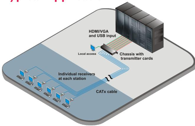
**Models** The CrystalView HDT is available in a single chassis model, which can host a combination of up to six HDMI or VGA Transmitter cards.
