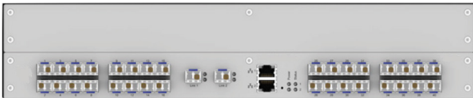
Fig.27 – 32 port, Fiber Matrix Grid, 2U
