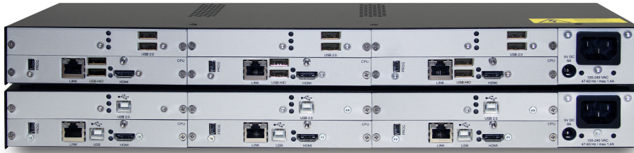
Figure 3. Various cards installed in six card chassis
