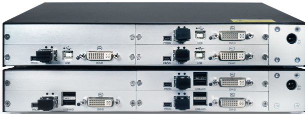
Figure 2. Various cards installed in four card chassis
