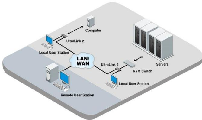
**Installation** The UltraLink 2 HDMI is easy to install and configure. Connect a display, USB keyboard and mouse to the local console ports, and connect the UltraLink 2 HDMI directly to a PC and a valid network. An OSD configuration window allows entry of IP address, DHCP, Net Mask, Gateway and Port access details. Video from the connected computer will be displayed on the local console's monitor, providing complete and secure control of the connected computer.
