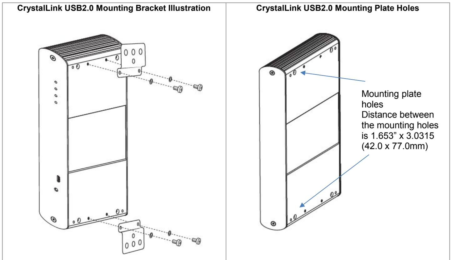
Figure 5. Chassis mounting options
