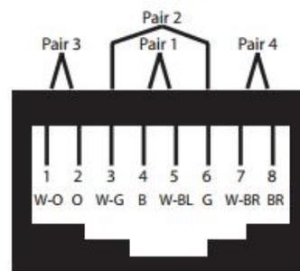
Figure 6. CAT5e/6/7 cable termination pinning
