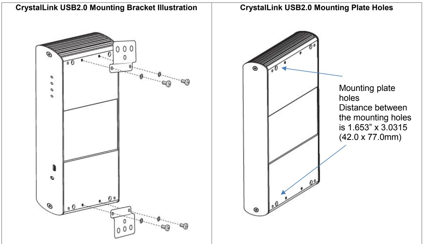
Figure 5. Chassis mounting options
