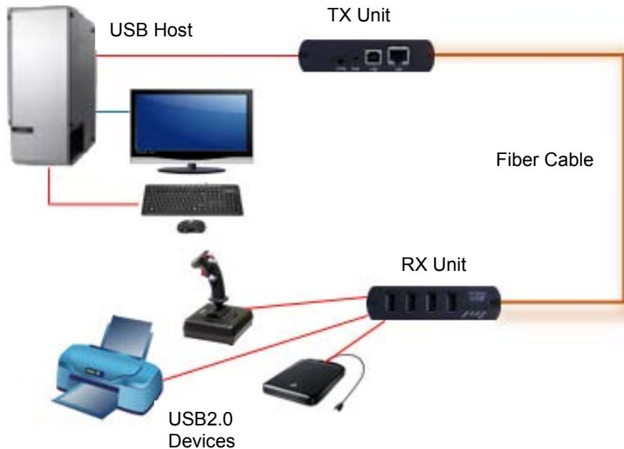
Figure 4. Crystallink USB2.0 fiber extender – standard installation
