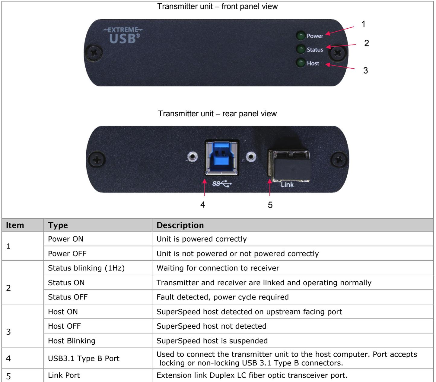
Figure 1. transmitter unit – LED's and connectors
