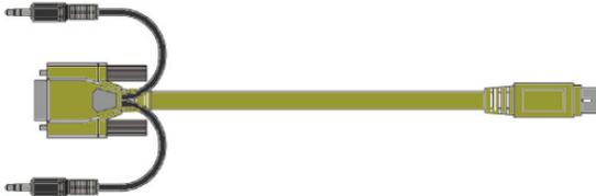
3. PS/2 Keyboard/Mouse "Y" cable. Mini-DIN 6(M) to 2\*mini-DIN 6(F). For connecting local keyboard and mouse to PS/2 equipped transmitter units.
