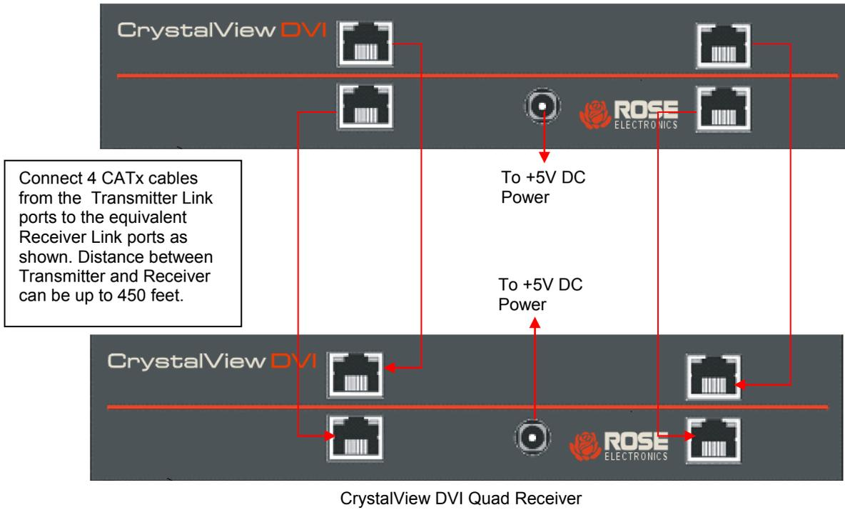
Figure 1. Connecting 4-port Transmitter and Receiver
