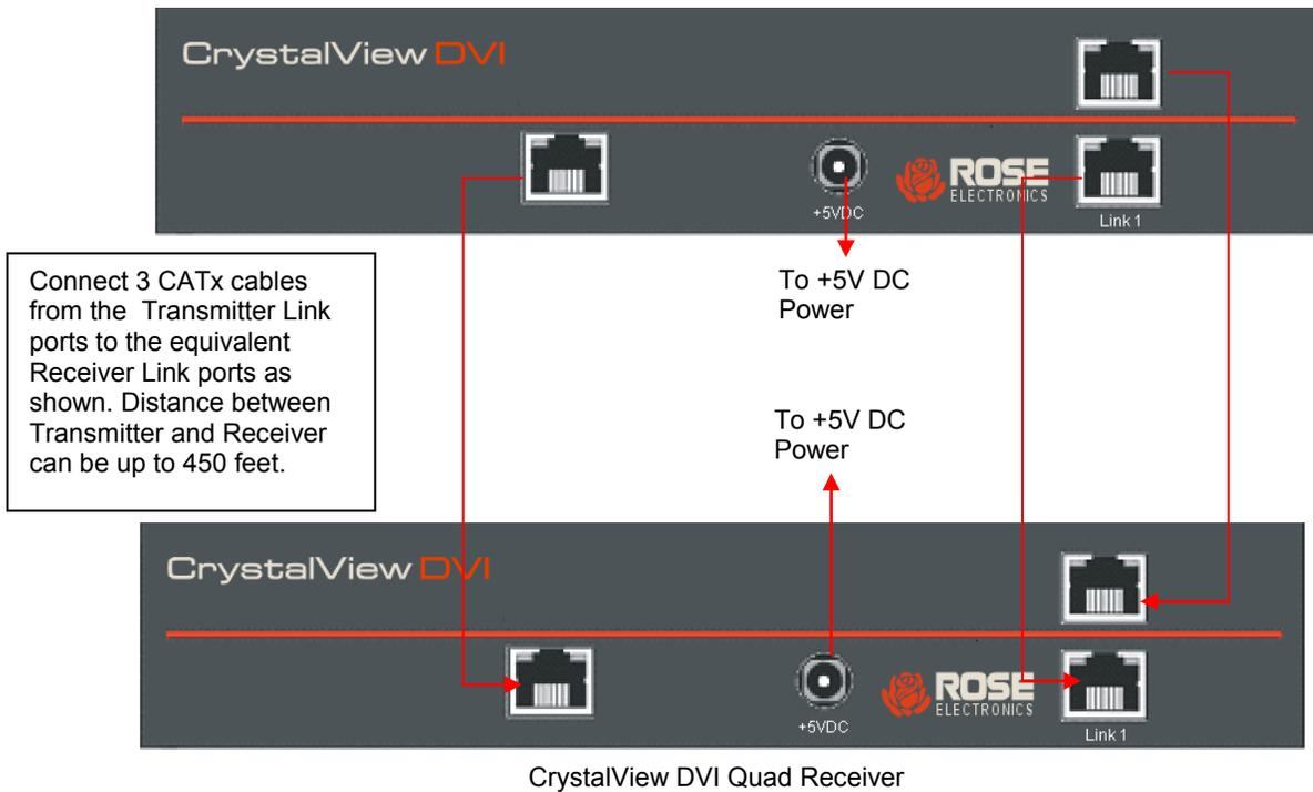
Figure 2. Connecting 3-port Transmitter and Receiver
