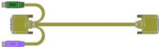
2. Serial / Audio Cable. DB9F + 2\*3.5mm audio to mini-DIN 8. For analog audio and serial equipped transmitter units.
