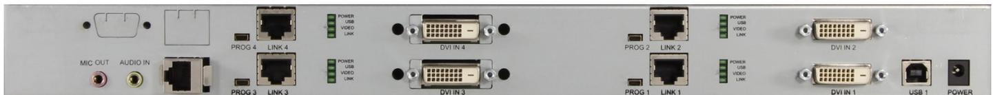
Figure 5. Sample CrystalView EX DVI Quad Transmitter Rear Panel
