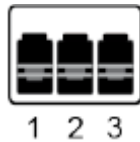
Figure 149. PCB 3-Pole Power Supply Connector Pinouts
