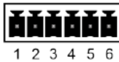
Figure 141. Phoenix Terminal Block, 6-pole Connector on Transmitter Pinouts
