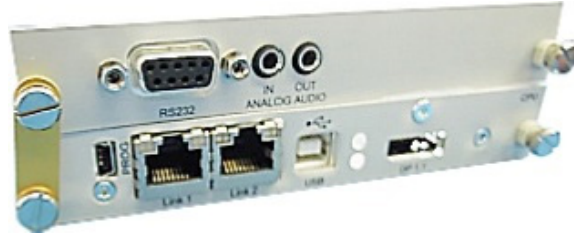
Figure 65. Paired Main Video Card and Option Card Joined with a Connection Plate
