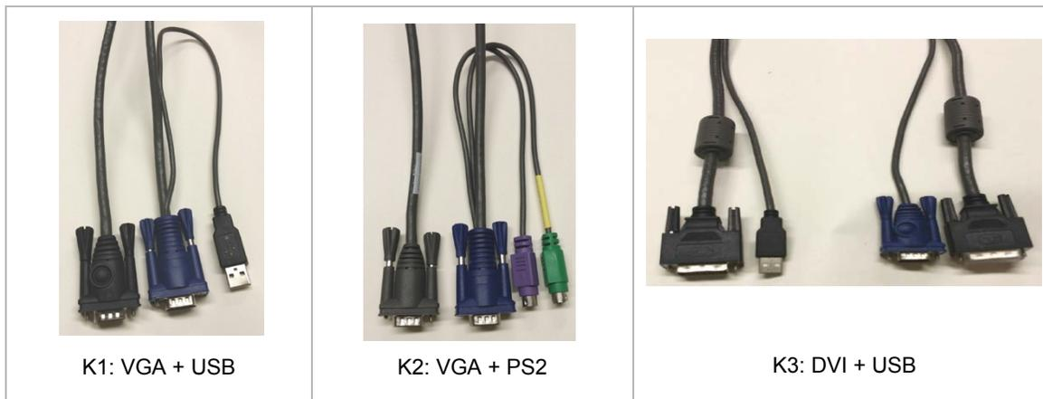
Figure 9. RackView device interface cables
